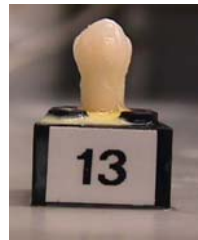
Premolar mounted on plastic block to allow precise positioning for repeat imaging
